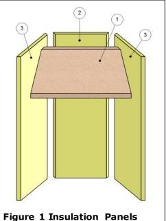
Figure 1 Insulation Panels and Fireplace Throat
