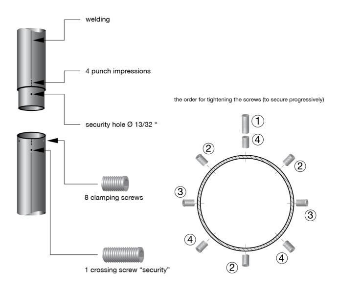
Note: the junction sleeves are manufactured only in case the floor to ceiling height in the room requires to manufacture the focus pipe in several parts (you may not find junction sleeves on usual ceiling heights).
