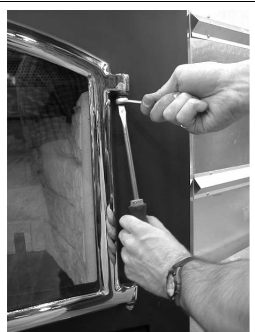
Figure 6 Door Hinge Adjustment
