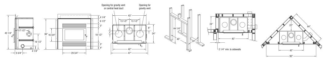
\* All RSF fireplaces can be installed directly on the combustible materials of the framing; the fireplaces are all zero clearance. The suggested framing dimensions are larger than necessary to facilitate the installation of the fireplace.
